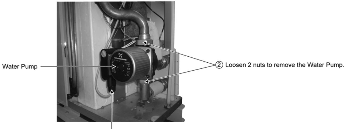
① Disconnect the connector of Water Pump.
