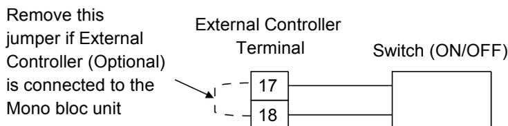
Diagram 4.2: External Controller connecting diagram
